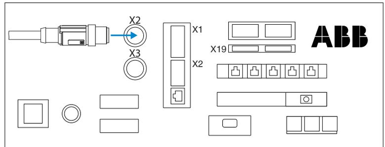
▶ Connect plug-in connector XG1 to connection X1.
