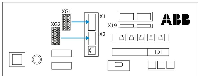
▶ Connect the plug-in connector connected to XG1 and XG2 to connection X19.
