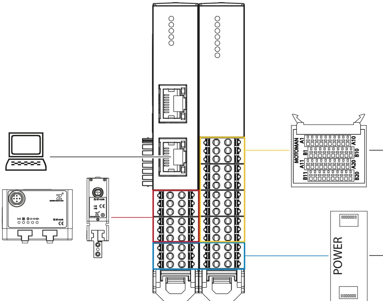
The standard wiring corresponds to the standard configuration in the Comfort App. If you do the standard wiring and keep the standard configuration in the Comfort App, your grippers will function with the robot.
