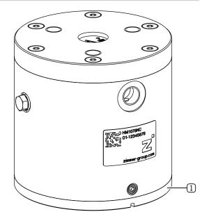
1 Demagnetized contact plate
