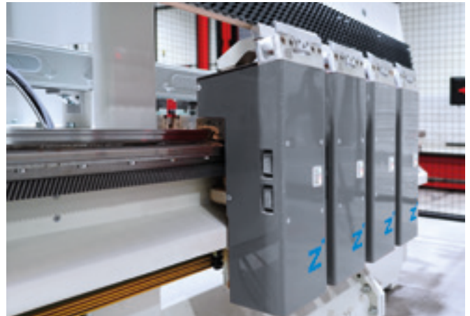
Transport system with circulating shuttles
