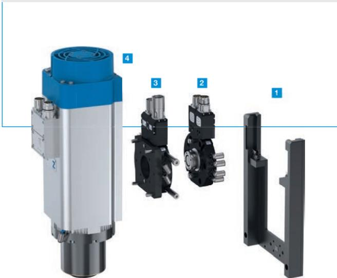
▶ Specially designed robot change units are available for motor spindles that are designed for use with robots. The robot change units provide a reliable interface between the robot and motor spindle. The loose part is attached to the motor spindle, while the fixed part is mounted at the end of the robot arm. A storage station is supplied to set the motor spindle aside when it is not being used.
